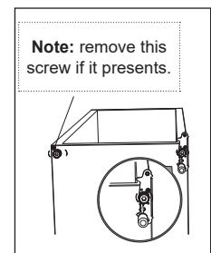
9. Unscrew and remove the bottom hinge pin, turn the bracket over and replace it.
