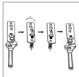
6. Refit the bracket fitting the bottom hinge pin. Replace both adjustable feet.
