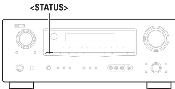
Information on the main unit's various settings (Status) and on input signals (Audio Input Signal) is shown on the display.
