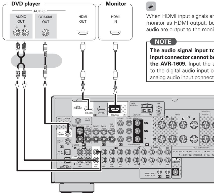
When HDMI input signals are sent to the monitor as HDMI output, both video and audio are output to the monitor.
