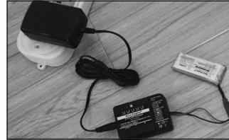
Connect the battery charger to the mains PSU, and plug the PSU into a mains socket. The red monitor LED on the charger lights up.
