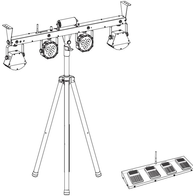
For mobile use place the light set on a lighting stand via the stand sleeve and fasten the fixation screw. Suitable stands can be found in chapter Accessories.
