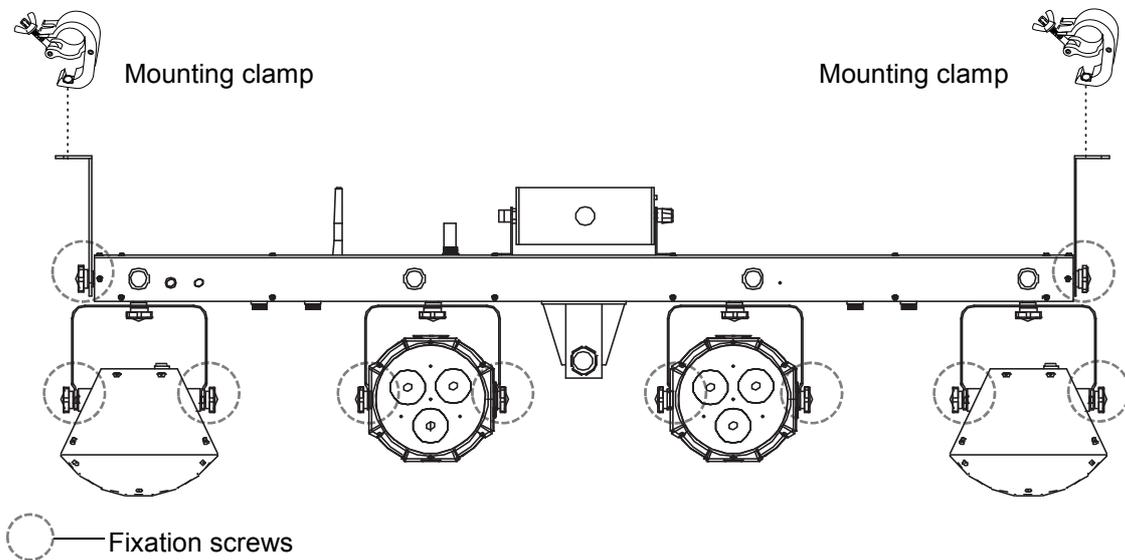
This product is designed for overhead rigging to a wall or ceiling with the mounting brackets. If necessary, it can also be fastened to a truss using appropriate clamps.
