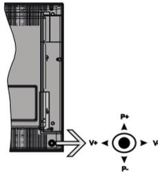
The joystick allows you to control the Volume / Programme / Source and Standby-On functions of the TV.
