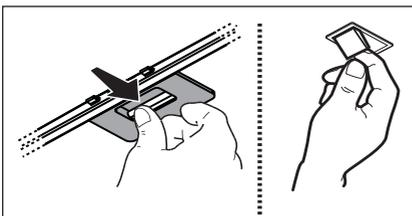
**4.2 NON-washable activated charcoal filter** - The saturation of the **charcoal filter** occurs after more or less prolonged use, depending on the type of cooking and the regularity of cleaning of the grease filter. In any case it is necessary to replace the cartridge at least every four months. The charcoal filter may NOT be washed or regenerated.
