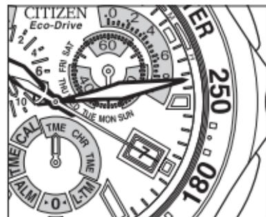
When radio waves have been received properly, the second hand returns to one-second interval movement and each hand is automatically corrected to the correct time. If radio waves were unable to be received, the watch returns to the time prior to radio wave reception. Never move the watch until the second hand returns to one-second interval movement.
