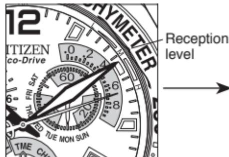
The second hand moves to either the H, M or L reception level. Although the second hand may turn to correct the time during reception, this does not mean that reception is completed.
