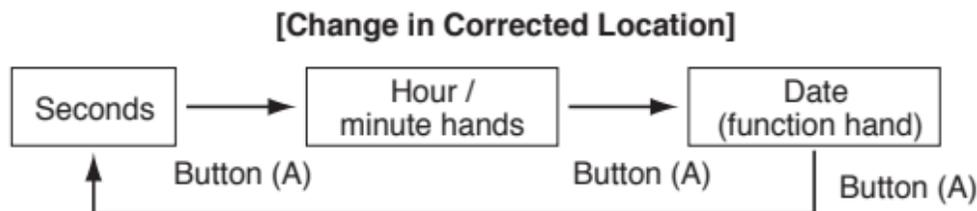
Pull the crown out to Position 1 and turn to align the mode hand at ►0◀ (reference position). When the crown is then pulled out to Position 2, the second hand advances continuously and then stops to indicate that the watch has entered the reference position correction mode.
