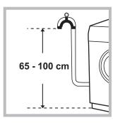
Connect the drain hose, without bending it, to a drainage duct or a wall drain located at a height between 65 and 100 cm from the floor;
