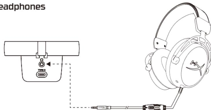
Connect headphones to the headphone jack on the microphone for microphone monitoring and playback audio.
