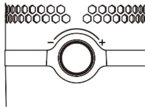
Push the multifunction button to switch between the microphone's two polar patterns, indicated by the LED ring.
