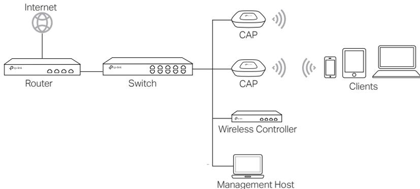
The wireless controller can be in the same or different subnet with the CAPs. And the management host is used to log in to the wireless controller to centrally manage the CAPs.
