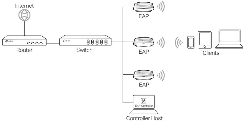
A computer running the EAP Controller software, which can be in the same or different subnet with the EAPs, is used to centrally manage the EAPs.
