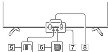
**[5] BUILT-IN MIC SWITCH\*<sup>2</sup>:** Turn on/off the built-in MIC.
