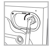
2. Connect the inlet hose to the washing machine by screwing it onto the corresponding water inlet of the appliance, which is situated on the top right-hand side of the rear part of the appliance (see figure).
