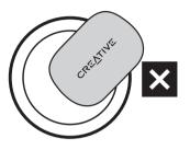
Creative Sensemore Air supports Qi-enabled wireless charging. To charge both the charging case and earbuds wirelessly, slot the earbuds into the case's magnetic charging slots, then place the charging case on the wireless charging pad \*. Do note that the earbuds cannot be charged wirelessly without its charging case.
