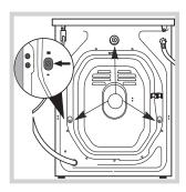
3. Remove the **3** protective screws (used during transportation) and the rubber washer with the corresponding spacer, located on the rear part of the appliance (see *figure*).
