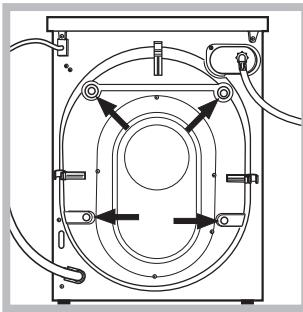
3. Remove the 4 protective screws (used during transportation) and the rubber washer with the corresponding spacer, located on the rear part of the appliance (see figure).
