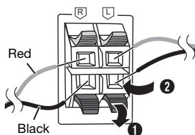
Be careful not to cross (short-circuit) or reverse the polarity of the speaker wires as doing so may damage the speakers.
