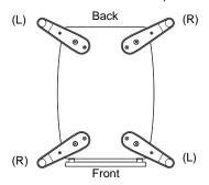
Use the 8 specified holes located on the base of the speaker.
