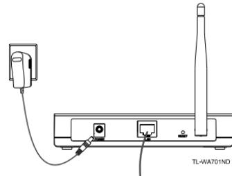
**Note** If the distance between the outlet and the Access Point is too long to supply the power, you can refer to the Power over Ethernet(PoE) solution in **Appendix B: With PoE Setup**.
