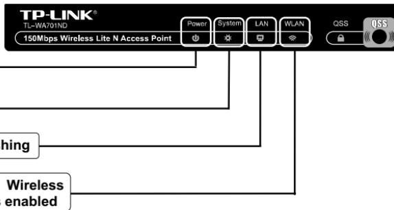
**Note** If the LEDs display abnormally, please check to see if all the cable connectors (power adapter and Ethernet cable) are well connected to your device.
