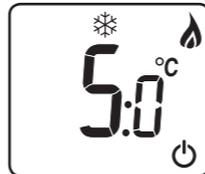
Frost protection is not available in cooling operation
