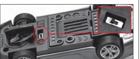
This is necessary and/or possible in case the running direction shall be changed. Therefore the reversing switch at the car's bottom side has to be positioned accordingly.
