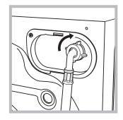
2. Connect the inlet hose to the washing machine by screwing it onto the corresponding water inlet of the appliance, which is situated on the top right-hand side of the rear part of the appliance (see figure).
