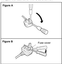
2. Replace the fuse and close or attach the fuse cover.
