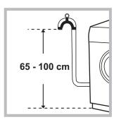
Connect the drain hose, without bending it, to a drainage duct or a wall drain located at a height between 65 and 100 cm from the floor;
