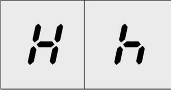
The hob has a residual heat indicator for each hotplate. It shows which hotplates are still hot. The residual heat indicator has two levels.
