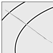
Scratches caused by salt, sugar or sand particles or from rough pan bases.
