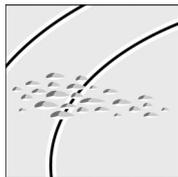
Blisters caused by melted sugar or food with a high sugar content.
