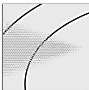
Shimmering metallic discoloration caused by pan abrasion or the use of unsuitable cleaning agents.
