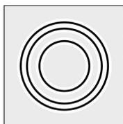
You can also switch on the medium and large filament circuits when using this hotplate. The hotplate must be switched on.
