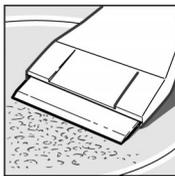
You can remove thick dirt best with a glass scraper.
