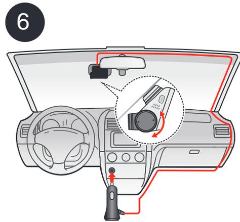
**CAUTION:** Connect the power source to the cradle for powering. Do not power the device from both the cradle and the Micro-USB connector on the device.
