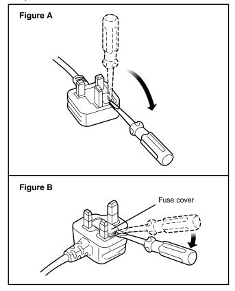
2. Replace the fuse and close or attach the fuse cover.
