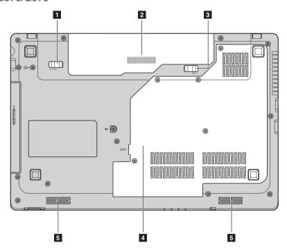
Battery latch -The manual battery latch is used to keep the battery pack 1 secured in place. manual For details, see "Using AC adapter and battery" on page Battery pack 12. The spring-loaded battery latch keeps the battery pack Battery latch -3 secured in place. spring loaded 4 Hard disk drive (HDD)/Memory/ **CPU** (Central processing unit)/ **Mini PCI Express Card slot** compartment 5 Speakers (Select The stereo speakers provide rich and powerful sound.
