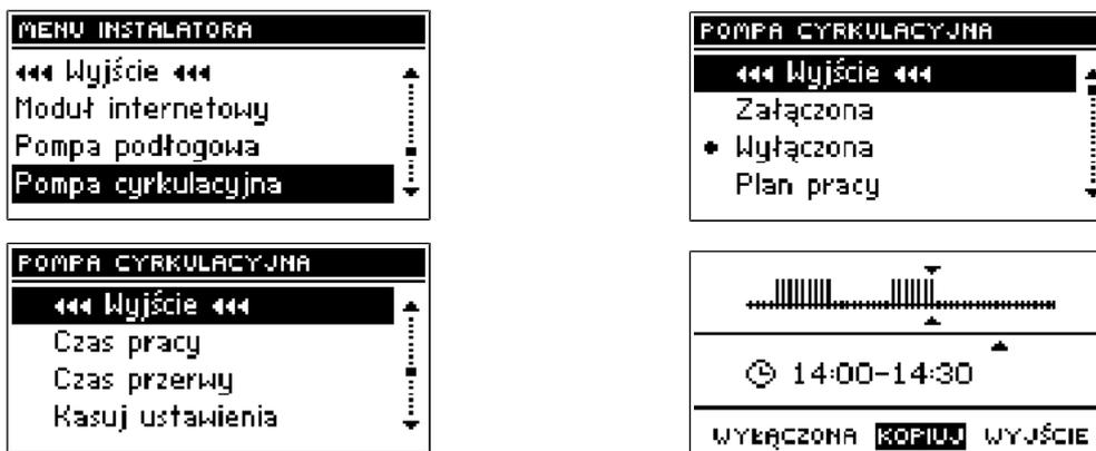
The function allows controlling the pump which is used to mix hot water between the boiler and the domestic hot water taps. After the function is activated the user sets the 24h activation cycle or pause cycle accurate to 30 minutes.
