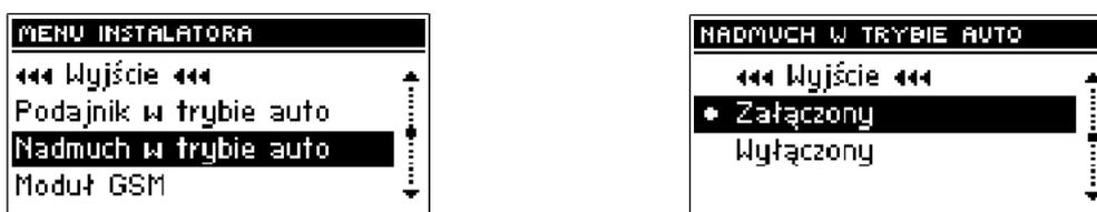
Automatic operation of the fan can be enabled or disabled using this function. Blowing can be disabled to manually control the natural chimney draught.
