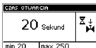
You can use this function to set the time for the full opening of the valve, that is to say, how long it takes to open the valve to 100%. This time should be selected according to your valve actuator (shown on the nameplate).
