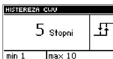
Use this option to set your set-point temperature hysteresis at the boiler tank. This is the maximum difference between the set-point temperature (your required temperature for the boiler tank when the pump turns off) and the temperature when its operation is to resume.
