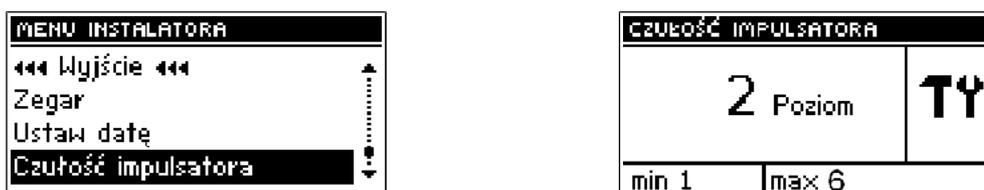
With this setting you can change the sensitivity of the pulsar knob within a range from 1 to 3 (where 1 means the highest sensitivity).
