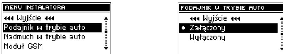
The option allows the automatic operation of the feeder to be enabled or disabled. The feeder can be disabled to feed fuel manually or to shut the boiler down.
