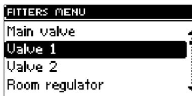
**NOTE:** Control with an additional valve (1 or 2) is only possible after you purchase and connect the controller to an additional control module (ST-61),
