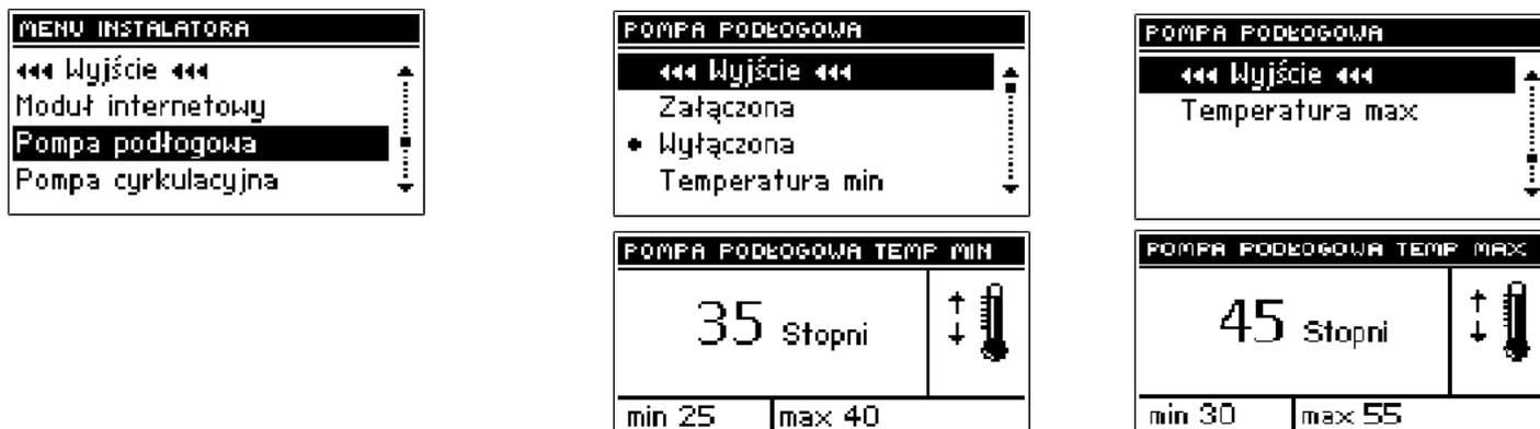
The function is used to control the floor heating. The user sets the floor heating temperature in the range between 30°C to 55°C. After activation of the floor pump the minimum activation (threshold) temperature (measured on the boiler) and the maximum (preset) temperature of the floor heating (measured on the pump sensor) should be set.
