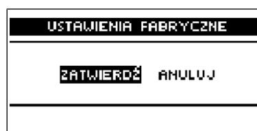
The controller is pre-configured for its operation. However, its settings should be modified to meet your individual needs. You can return to the factory settings at any time. If you enable the **factory settings** option you will lose all of your own boiler settings, which will be replaced with the settings saved by the boiler manufacturer. From now on you can re-set your own parameters of the boiler.
