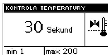
This parameter determines the sampling (control) frequency of the water temperature downstream of the valve for the central heating or hot water system. If the sensor indicates a change in temperature (deviation from set-point), then the solenoid will open or close partially by a preset step to restore the set-point temperature.
