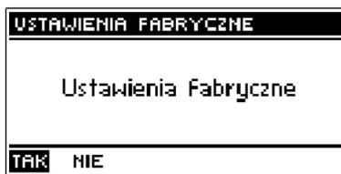
This parameter allows you to restore the mixing valve settings saved by the manufacturer. By restoring the factory settings you will not change the valve type setting (central heating or floor type).
