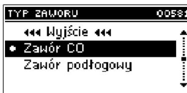
You can use this option to select the type of valve: central heating or floor type.
