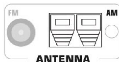
Place the antenna on a shelf or hang it on a window frame and turn it in the direction which gives the best reception. Keep all other wires such as power cords, speakers wires or interconnect wires as far away as possible from the antenna.
