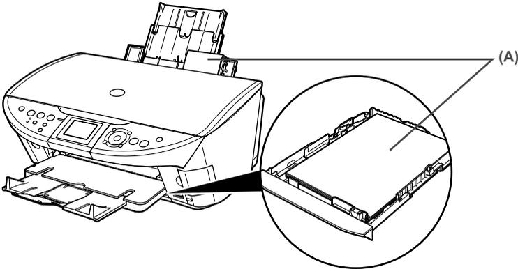
(A) You can switch between paper loaded in the Auto Sheet Feeder (e.g., 4" x 6" / 101.6 x 152.4 mm) or the Cassette (e.g., A4/Letter-sized paper).
