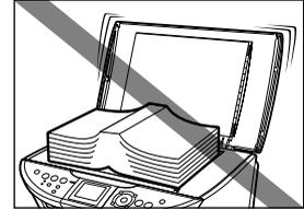
Do not place the following objects on top of the machine. If such objects come into contact with internal electrical components, the machine may short-circuit, resulting in fire or electrical shock.
