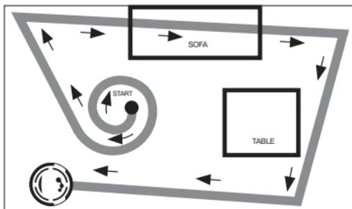
Vileda Cleaning Robot can avoid obstacles and is equipped with cliff sensors to avoid falling down the stairs.
