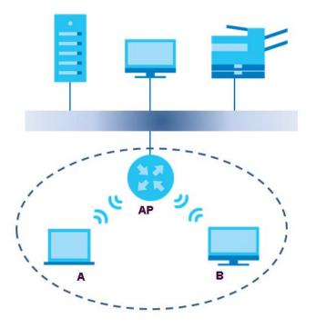
The wireless network is the part in the blue circle. In this wireless network, devices **A** and **B** are called wireless clients. The wireless clients use the access point (AP) to interact with other devices (such as the printer) or with the Internet. Your LTE Device is the AP.
