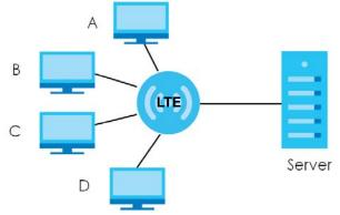
In the multicast example above, systems **A** and **D** comprise one multicast group. In multicasting, the server only needs to send one data stream and this is delivered to systems **A** and **D**.
