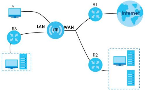
Figure 71 Example of Static Routing Topology
