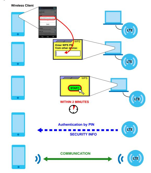
Figure 25 Example WPS Process: PIN Method
